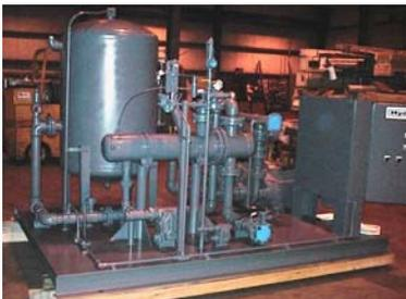
**Packaged pump and control skid.** Pumps, electrical enclosure, vent and surge tank, piping, valves, gauges, wiring and thermostatic modulating valves (if required), and the heat exchanger are all completely factory assembled on a structural steel frame with a solid steel base plate.
