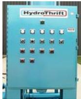
**Automatic control.** The NEMA 12 electrical enclosure contains motor starter(s) with overload and short-circuit protection, thermostatic controls, and an on-off selector switch for the circulating pump motor(s). The control circuit includes a control transformer for 110/1/60 and a power-on light.
