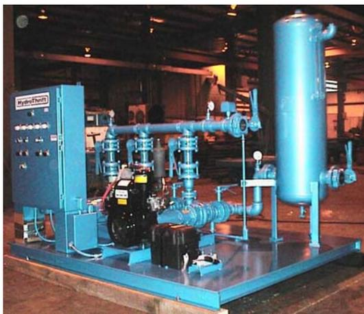
**Packaged pump and control skid.** Pumps, electrical enclosure, vent and surge tank, piping, valving, gauges, wiring and thermostatic fan control are all completely factory assembled on a full-deck fabricated steel base.
